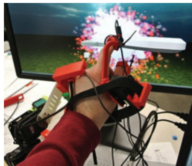
Figure. Left: Wrist exoskeleton with gripper interfaced with VE. Right: VE simulation in Unity of pinch task
