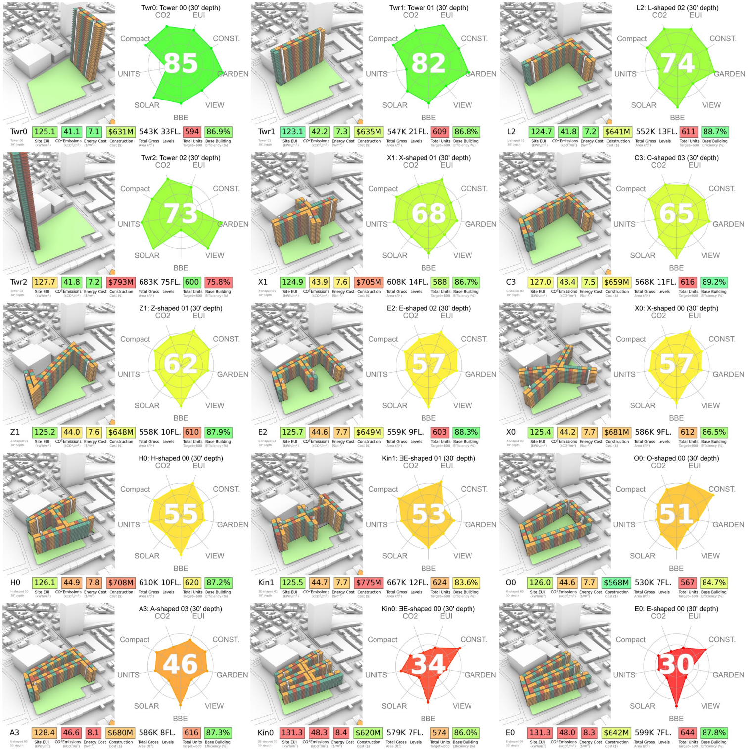
PCA visualizations of 52 layouts based on their performance scores in nine criteria from radar charts as their features. The color of a marker is based on the average score of all criteria from each layout (green being higher and red being lower).
