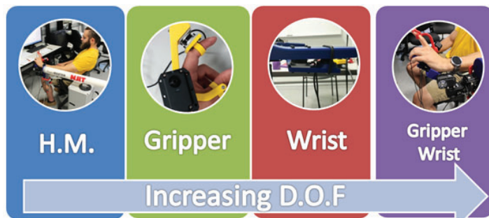
Figure. Experimental groups for Pick and Place Task in order of increasing DOF. All groups use Haptic Master( HM) with the respective DOF.
