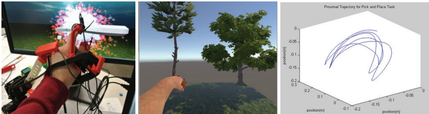
Figure. Left: Wrist exoskeleton with gripper interfaced with VE. Right: VE simulation in Unity of pinch task. Figure. Proximal arm trajectory evaluated with the Haptic Master
